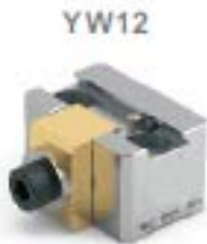
Dimension: 21*32*19mm Dovetail depth: 2.54mm Clamping range: 12-25mm Material: stainless steel Max. torque: 8Nm Weight/Kg: 0.15KG
