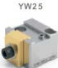
Dimension: 38*38*27mm Dovetail depth: 2.54mm Clamping range: 25-70mm Material: stainless steel Max. torque: 10Nm Weight/Kg: 0.25KG
